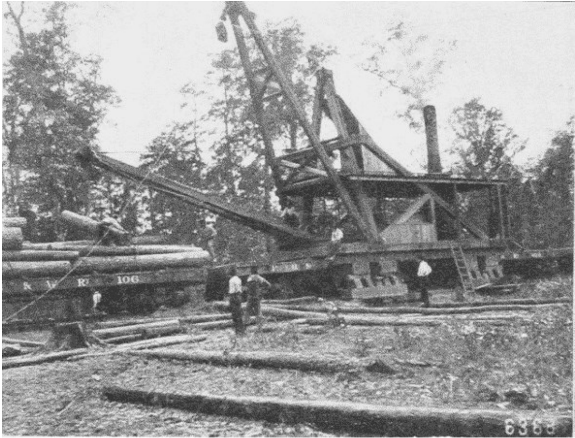
Fig. 27. Steam Skidder at Work. Grant County, Arkansas.
