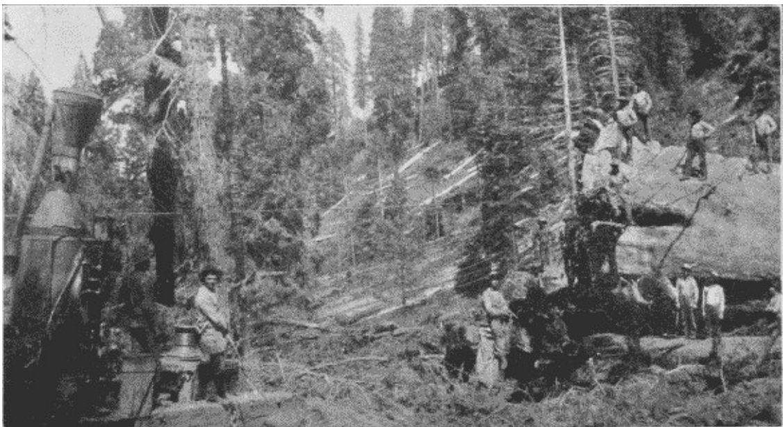
Fig. 26. Hauling Big Logs by Donkey Engine.
