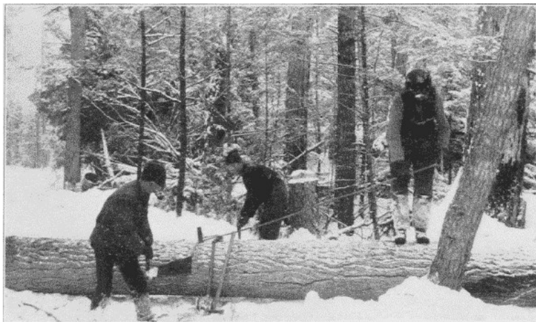
Fig. 6. Sawing Logs into Lengths.
