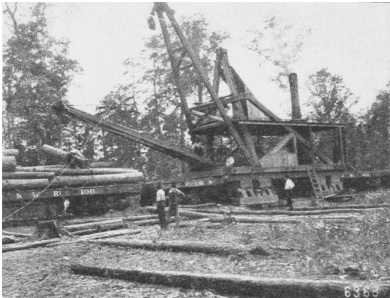
Fig. 27. Steam Skidder at Work. Grant County, Arkansas.
